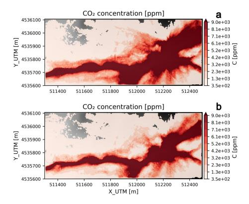
Long-term hazard maps of  $CO_2$  concentration at (a) 0.5 m and (b) 2 m above the ground averaged over the whole duration of the simulation (4 hours) at an exceedance probability of 5%.
